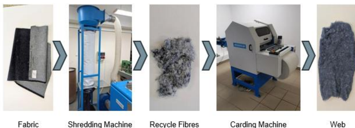
Figure 14. Technological system of TUL for mechanical recycling of cotton
